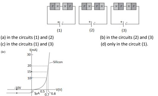
The V-I characteristic of a diode is shown in the figure. The ratio of the resistance of the diode at I = 15 mA to the resistance at V = -10 V is
